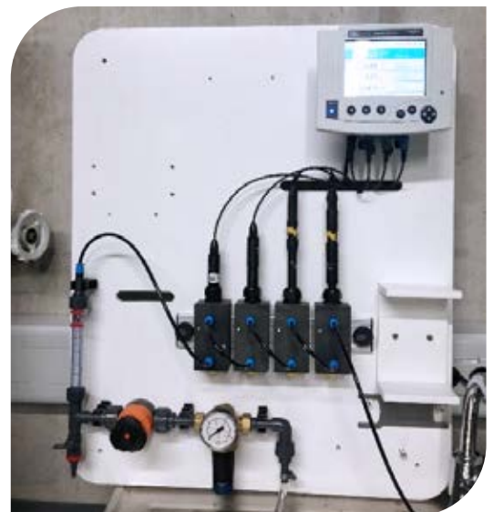
Fig. 3: Test bench for the WTW Drinking Water Panel at the Mörscher Wald waterworks near Karlsruhe with IQ SENSOR NET system 2020 3G and four IDS sensors
